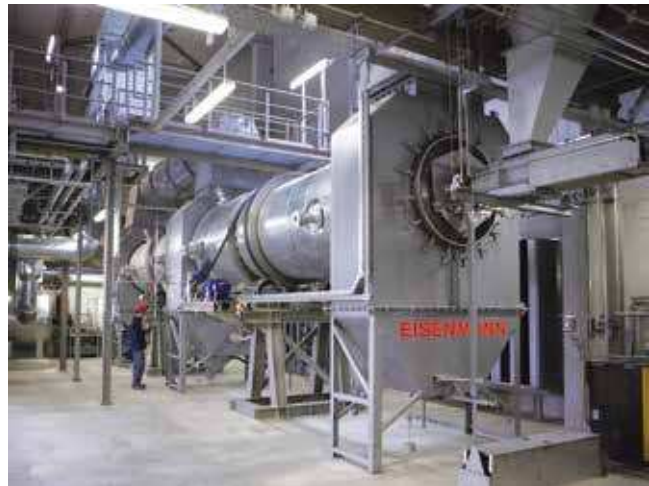
Rotary kiln for the treatment of hazardous waste
