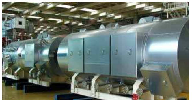
Combustion chamber for VOC treatment
